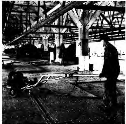
Portable electric reaming tool at work.
